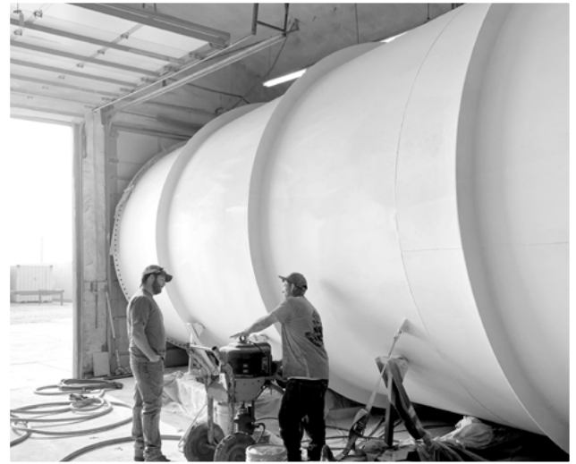
Dome Technology is building a second dome, pictured on the left, for American Crystal Sugar in Montgomery, Illinois, USA. Above: The tube gallery connecting the domes was fabricated at the Dome Technology shop in Idaho Falls, Idaho, USA.
